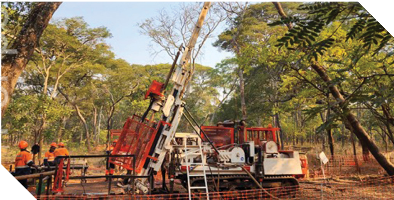
Figure 5. Phase 1 Diamond drilling rig on site at the Mumbhezhi Copper Project
