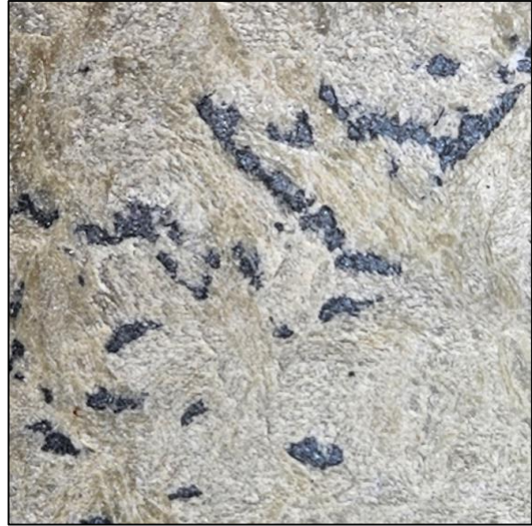
Figure 3: Coarsely disseminated tetrahedrite (copper – antimony sulphide) in massive siderite and barite veining. Drill core from BPD08.
