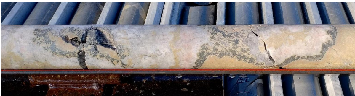
Figure 4: Drill core from BPD09 (about 223.5m down-hole depth) showing siderite (cream) and barite (white) veining. Abundant grey tetrahedrite is rimming colloform siderite-barite veining.
