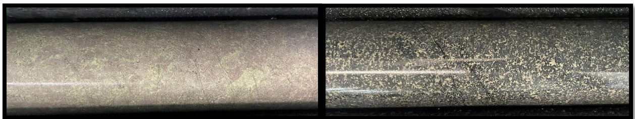
Figure 1. Typical sulphide mineralisation intersected in OVD021: hypogene massive sulphides comprising pyrrhotite-pentlandite-chalcopyrite at ~110m downhole (left) and matrix/net textured pyrrhotite-pentlandite-chalcopyrite at ~118m downhole (right).
