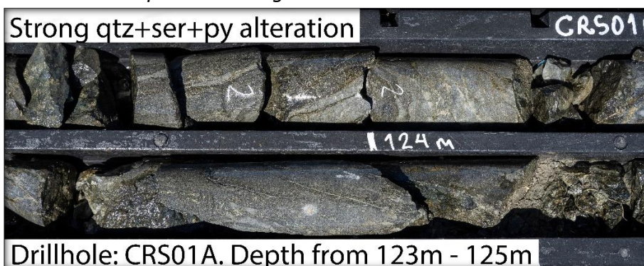
Photo 4. Core photo showing mineralisation in the Drillhole CRS01A
