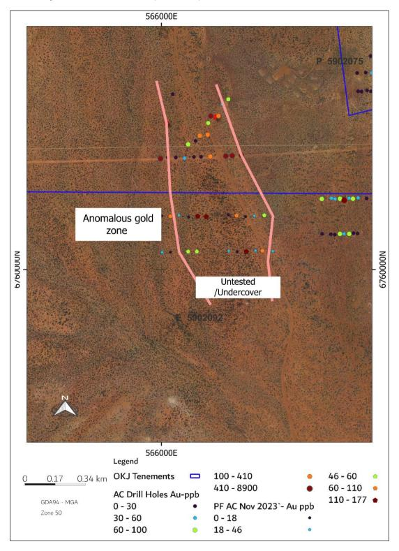
Figure 4: Paynes Find south Interpreted gold zone with AC drill holes and historic drilling coloured by gold ppb arial image.
