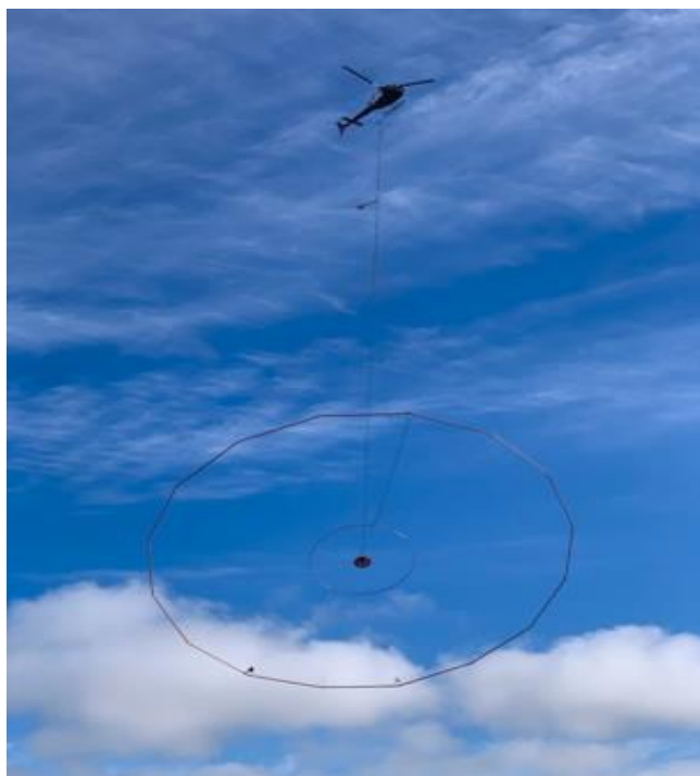
Figure 6: Helicopter with VTEM survey sensor array over the Lort River Project.
