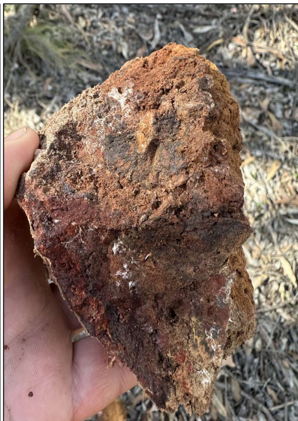
Figure 9 – Silver-Base metal mineralisation within gossan yielding 36.8 g/t Ag , 0.3% Cu-Pb-Zn & 0.2% Ba from sample 3000766
