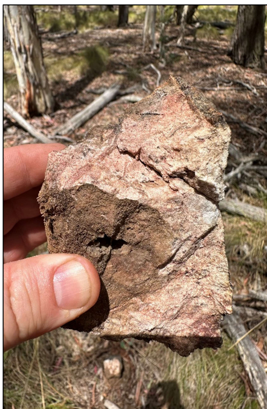
Figure 13 – Silver mineralisation within ferruginous sandstone yielding 318 g/t Ag, 0.37% Ba from sample 3000298
