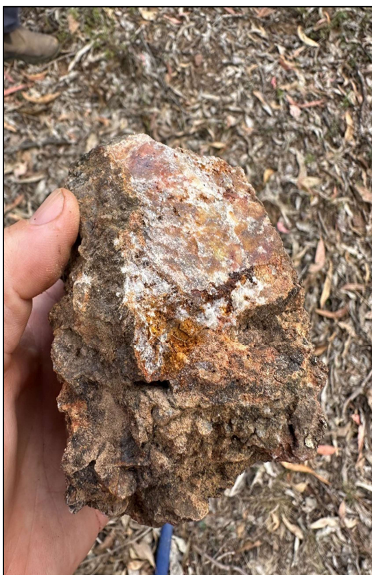
Figure 14 – Silver mineralisation within ferruginous quartz yielding 183 g/t Ag, 970 ppm Ba from sample 3000551
