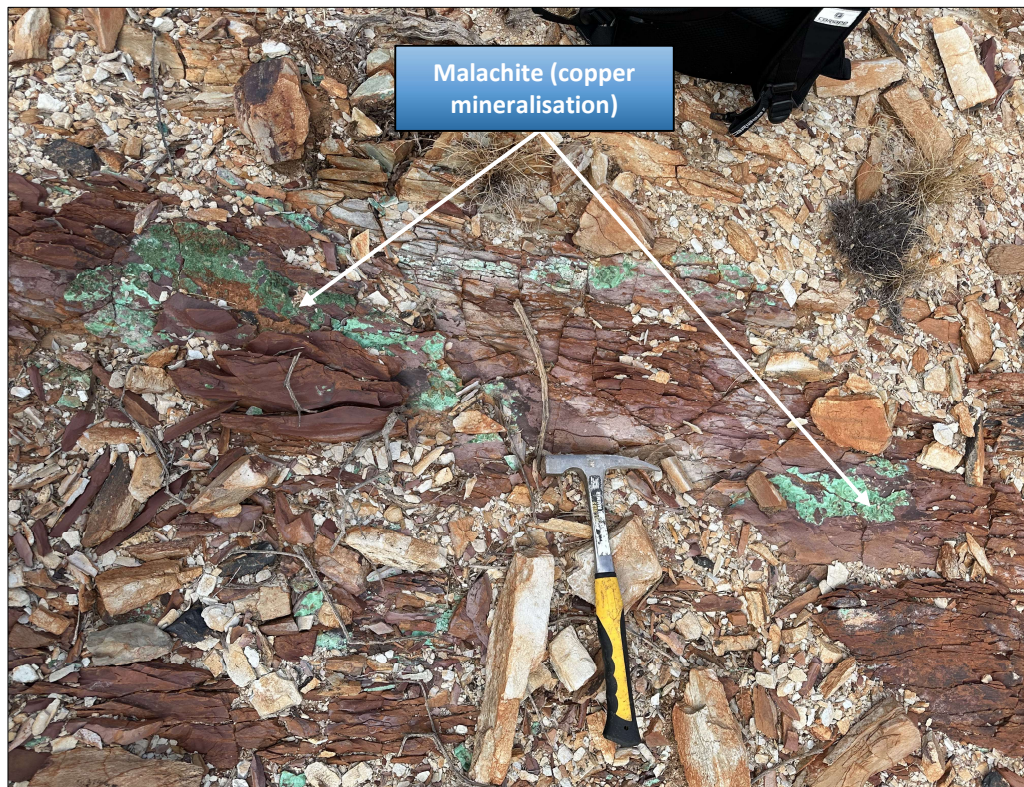
Figure 21 – Rock Chip Sample CH213 - Malachite eastern edge of 8-10m copper zone, strike 160° dip -30. Assay Results: 8.64% Cu
