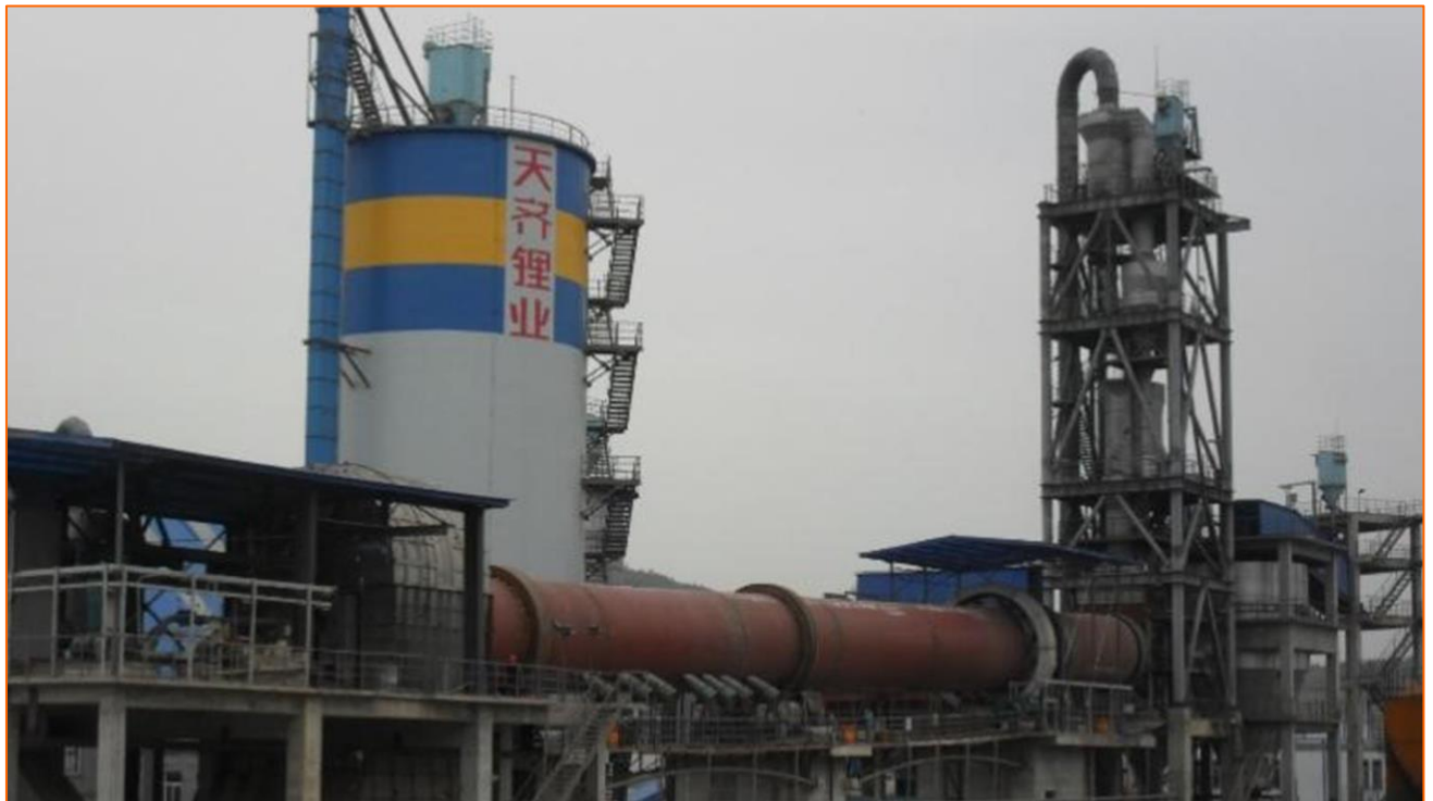
Figure 6: Typical natural-gas fired calcination kiln used in the lithium refinery process. Source: Sichuan Calciner Technology Pty Ltd
