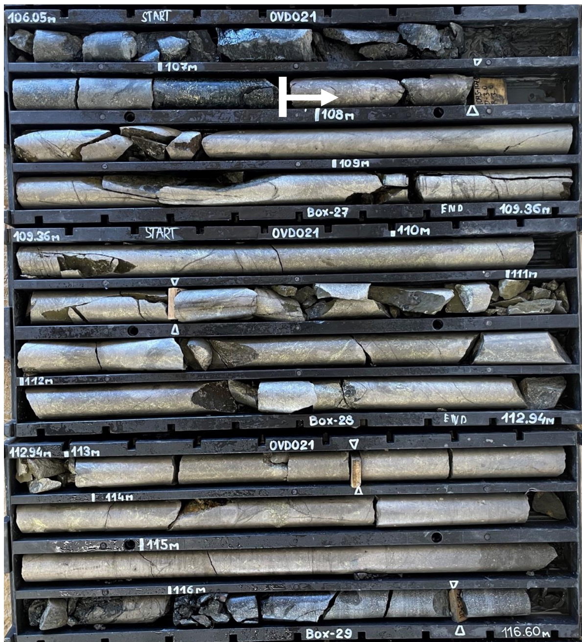
Figure 3: Drill core from OVD021, massive sulphide between 107.2m and 116m
