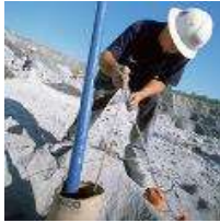
End-of-Hose device patented, allowing all gassing to take place in the borehole
