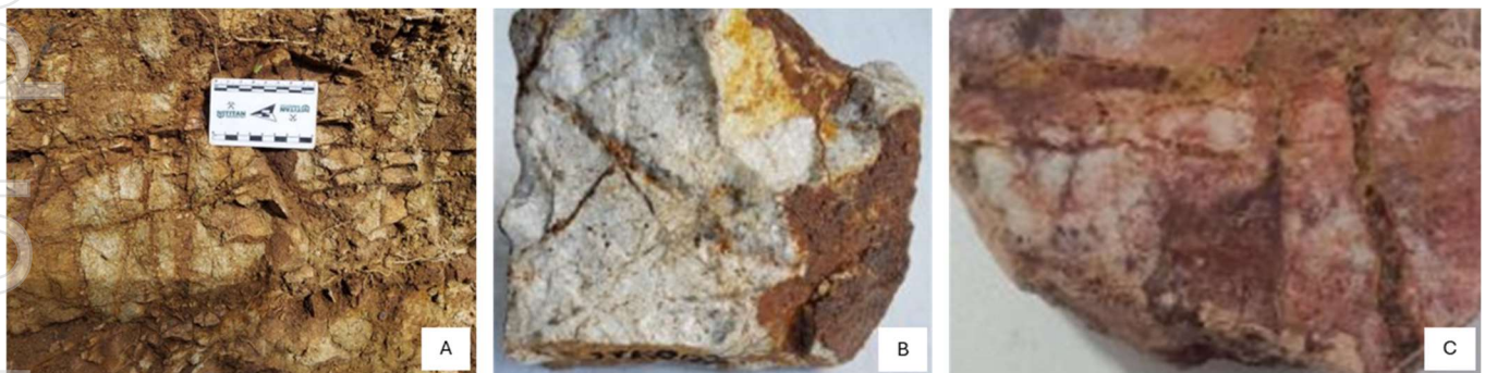
Plate 1. Trench and hand specimens taken from the Gisell prospect. A: Oxidised sulphide (iron oxide) veins in trenching. B: A-type vein in trenching. C: Oxidised sulphide (iron oxide) veins with irregular boxworks texture.
