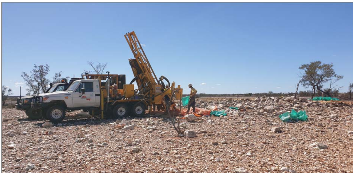
Photo 2. Aircore drill rig at the Bellagio Gold Prospect, with the main quartz vein outcrop shown to the right of the drill rig. Photo direction looking north east.
