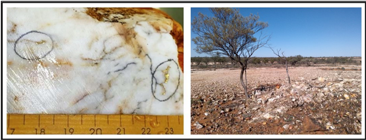
Photo 1. Visible Gold (circled) in historical sample of cut quartz vein (left) from outcrop (right). Scale of slab is in centimetres. Outcrop photo is looking west.
