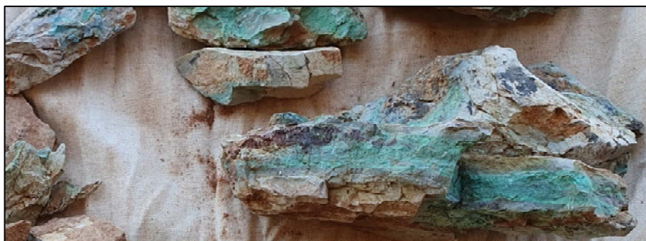
Photo 4. Rock chip sample from site KB03113 (2019), previously reported as 15.3% Copper , comprised of oxidized white meta-tuffaceous siltstone with oxide copper mineralisation (teal/green in photo).
