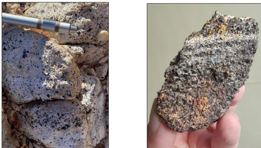
Photo 2 – Left – Typical outcrop of HMS titanium ore (dark minerals) in white silts. Right – high-grade ores (>30% TiO 2 ) from the Rosewood Prospect. The brown-black minerals are the Titanium-bearing mineral ores comprising ilmenite, leucoxene and rutile.
