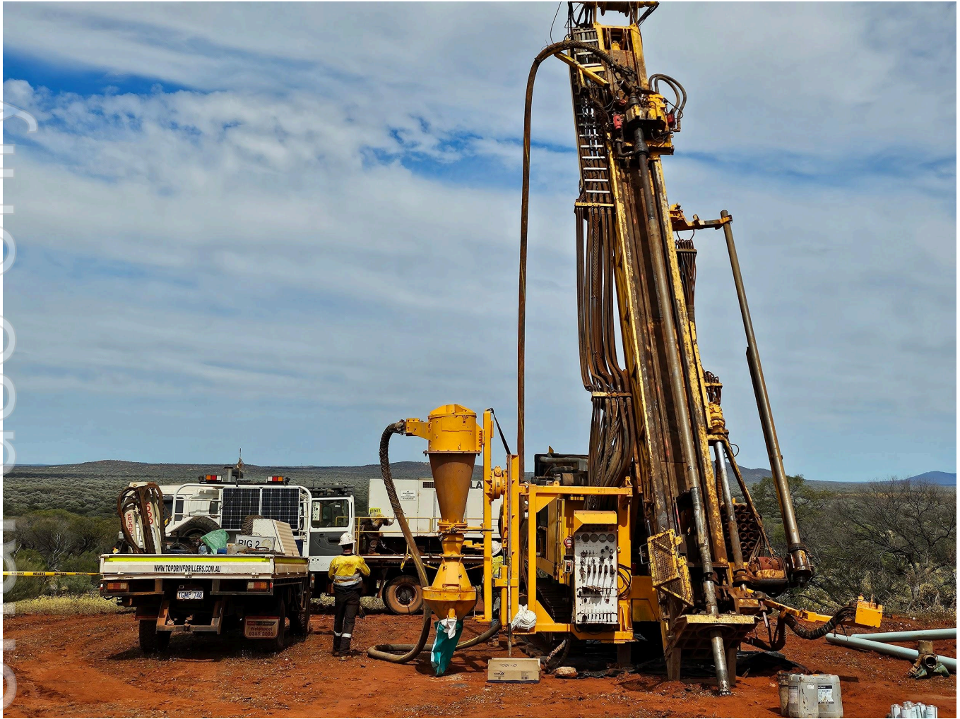
Figure 01: Reverse Circulation Drilling commencing on WARDH160 at the Remorse Target
