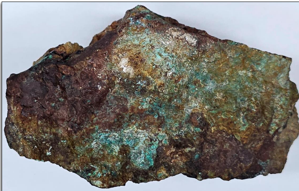
Figure 3: Sample AR28585, Piper prospect. Assays of 11.5% Cu, 18.8 g/t Ag and 1.1% Sb. Sample is ~400m north of quartz breccia outcrop. Sample is 14cm in length.
