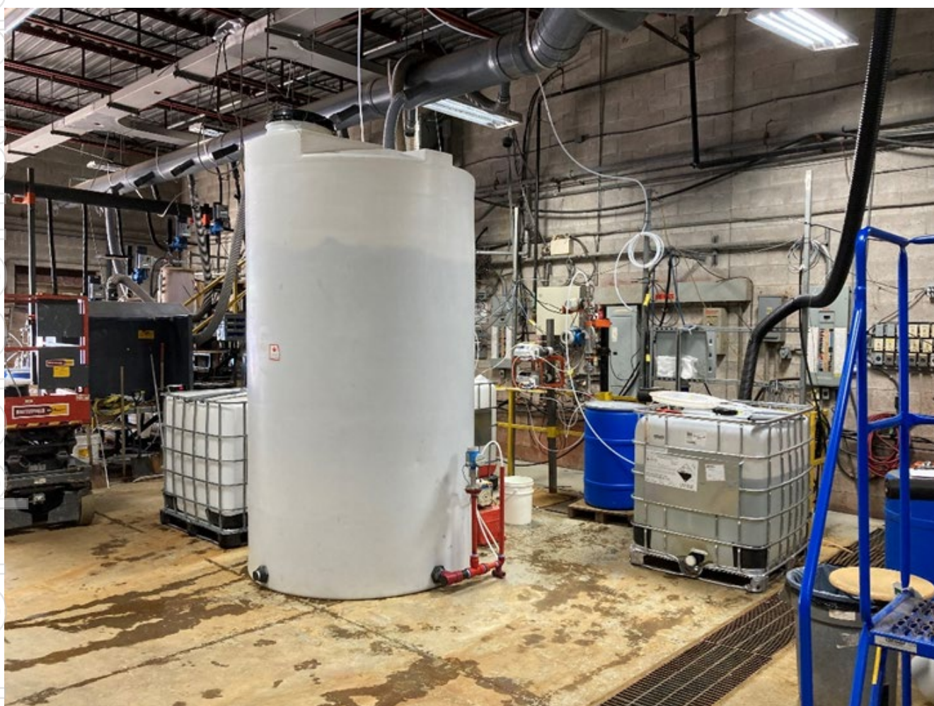
Figure 2: Bulk column of ore being leached, with Pregnant Liquor Solution collected and ready for the neutralisation and refining stage.
