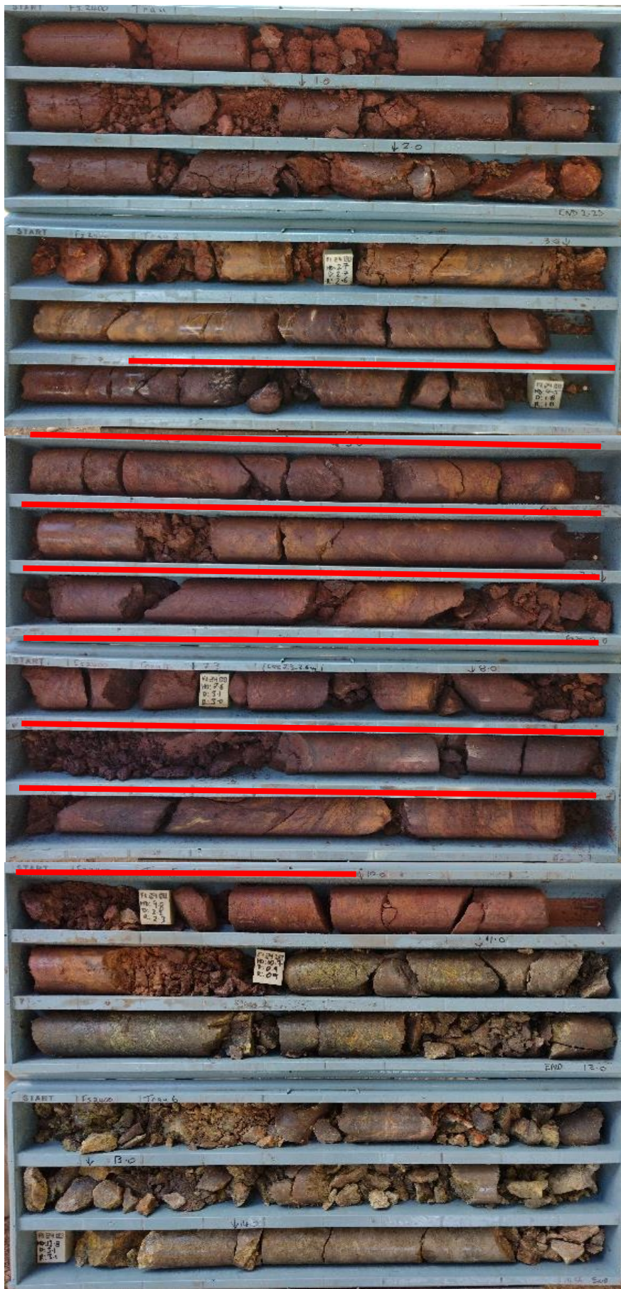
Figure 6 Melrose Mineralised Laterite Drillhole FI2400 0-15m
