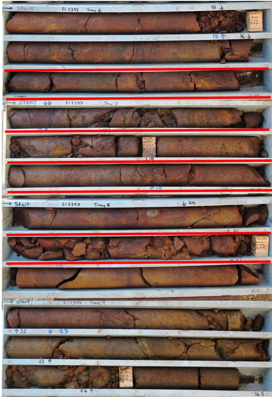
Melrose Mineralise Laterite Drillhole FI2397 14 to 24.5m
