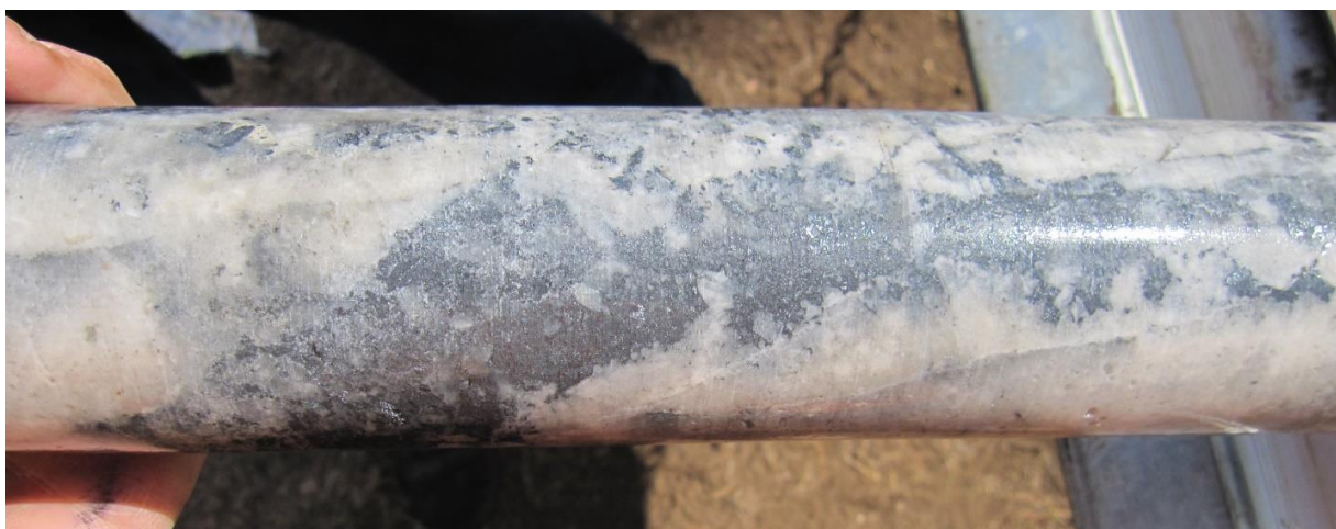
Figure 7: Banshee Antimony (Stibnite) Mineralisation in quartz (from drill hole CNDD01 89.90m to 90.20m approx.)
