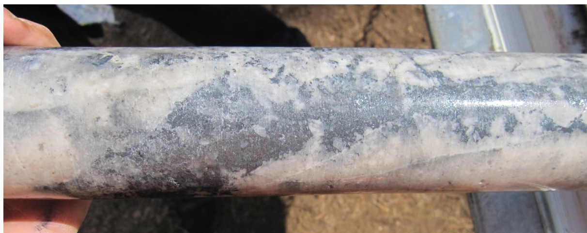
Figure 7: Banshee Antimony (Stibnite) Mineralisation in quartz (from drill hole CNDD01 89.90m to 90.20m approx.)
