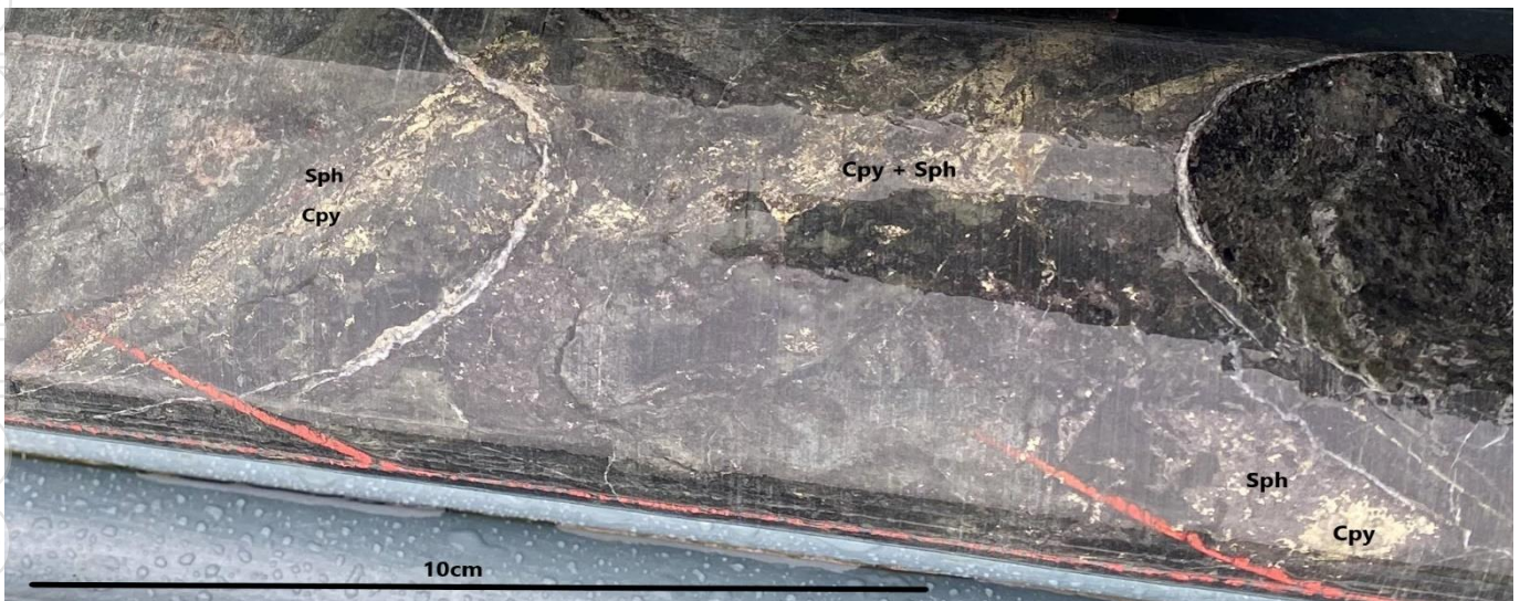
Image 1: HVD003, 85.8m to 86m: semi-massive sulphide patches of copper sulphide - chalcopyrite (cpy) and zinc sulphide - sphalerite (sph) in Ordovician mafic volcanics (pXRF readings up to 18.5% Cu, 34.8% Zn* – see Appendix 3)
