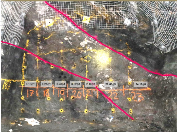
Ulysses underground - High grade ore development underway
