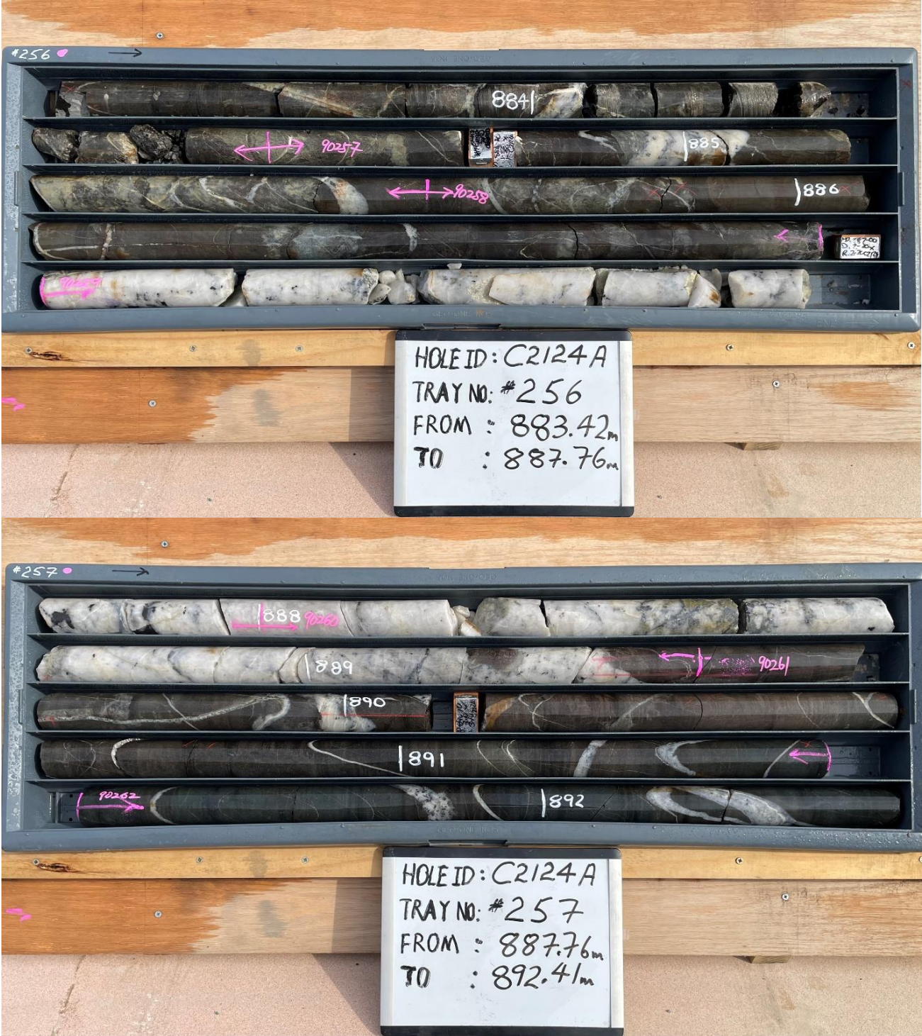
Figure 3. Mineralised quartz vein in drill hole C2124A from 887.0 – 889.4m
