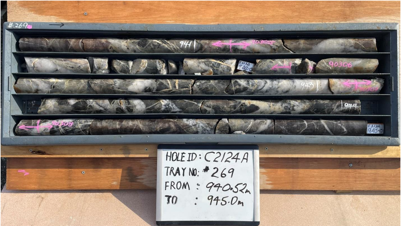
Figure 4. Mineralised quartz/sediment breccia within drill hole C2124A from 940.5 to 945.0m
