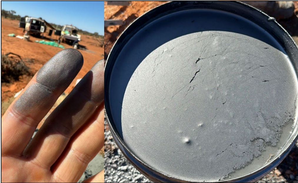
Figure 3: High grade graphite NY001RC at 252m depth (end of hole) – the “smear test” and “float test” assist grade & flake size estimates during visual logging of reverse circulation samples.
