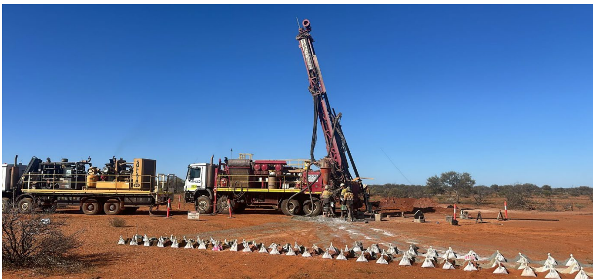
Figure 1: Reverse Circulation drilling at the Ranger Prospect, August 2024.
