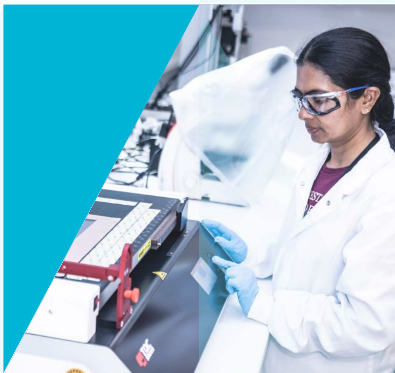
Madhavi Chagalamarri, Laboratory Technician sheet coating with anode formulation
