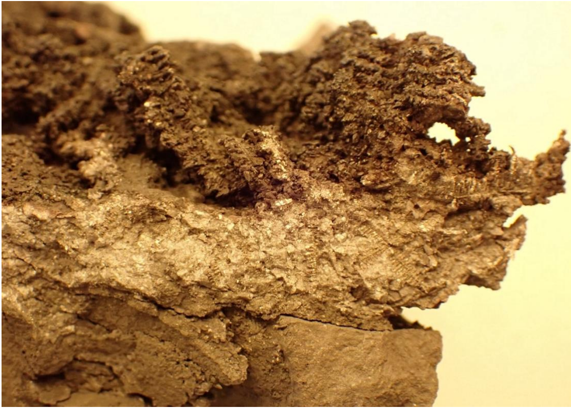
Figure 3 – Photograph of abundant native silver mineralisation in sample F005909 showing both tarnished and fresh silver within a calcite-chlorite matrix.
