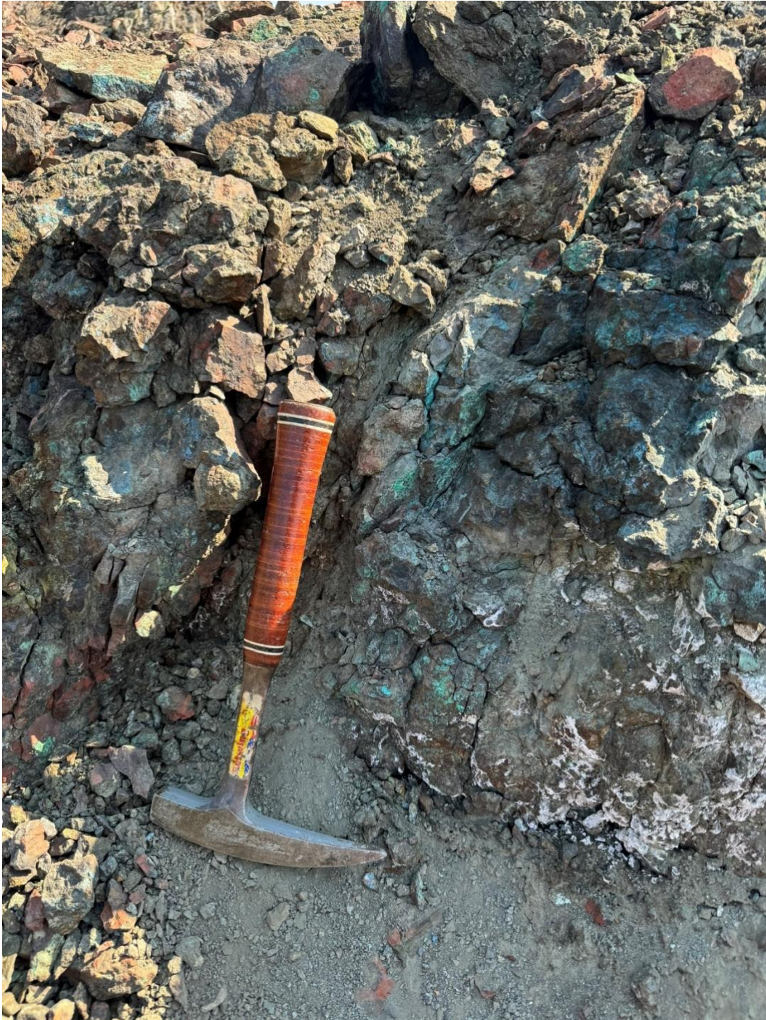
Figure 8 – Outcrop photograph for sample F005408 illustrating a brick red K-feldspar-skarn breccia with abundant copper secondary minerals after chalcopyrite-bornite-chalcocite sulphides. Sample returned 233g/t Ag, 9.82% Cu, 1.67% Pb, 2.35% Zn .
