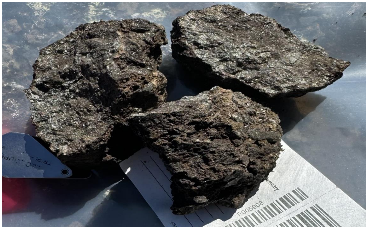
Figure 6 – Photograph of sample F005908, an intensely chlorite altered diorite with disseminated and vein hosted native silver which returned 9,070g/t Ag.
