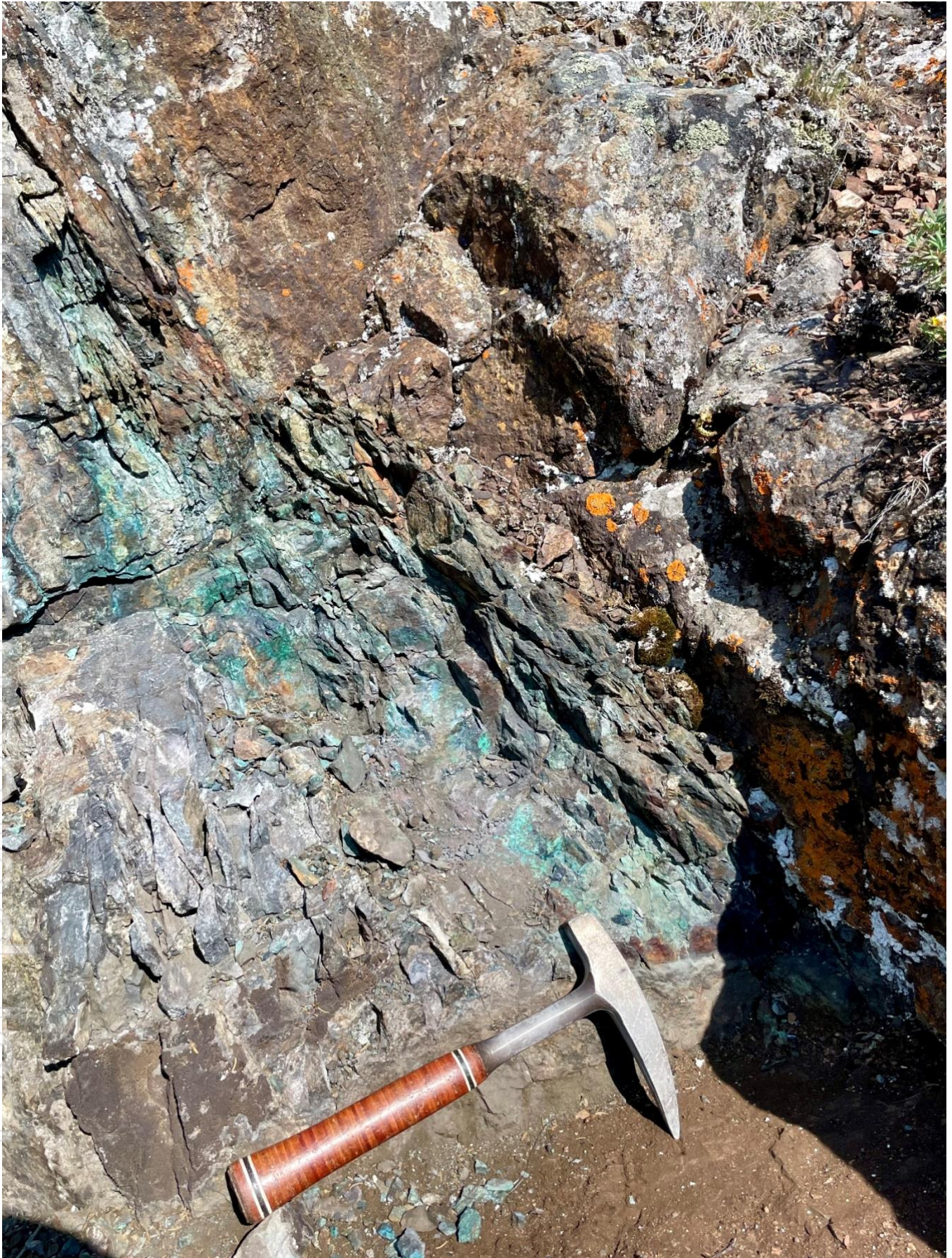
Figure 7 – Photograph of outcrop for sample F005606 which returned 904g/t Ag, 6.5% Cu and 8.06% Zn from the Spud Bonanza E/W trend.
