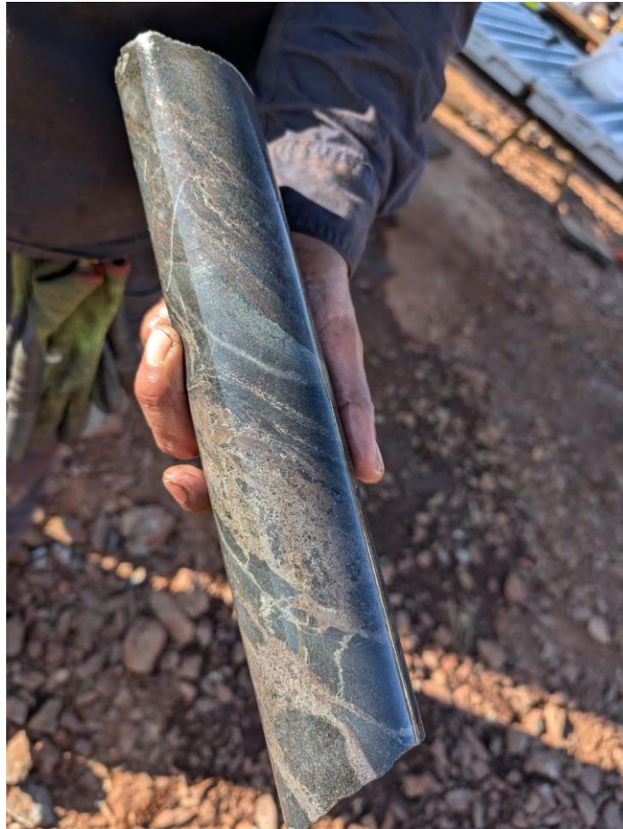
Figure 3: Sphalerite, galena and minor chalcopyrite in 24AED003
