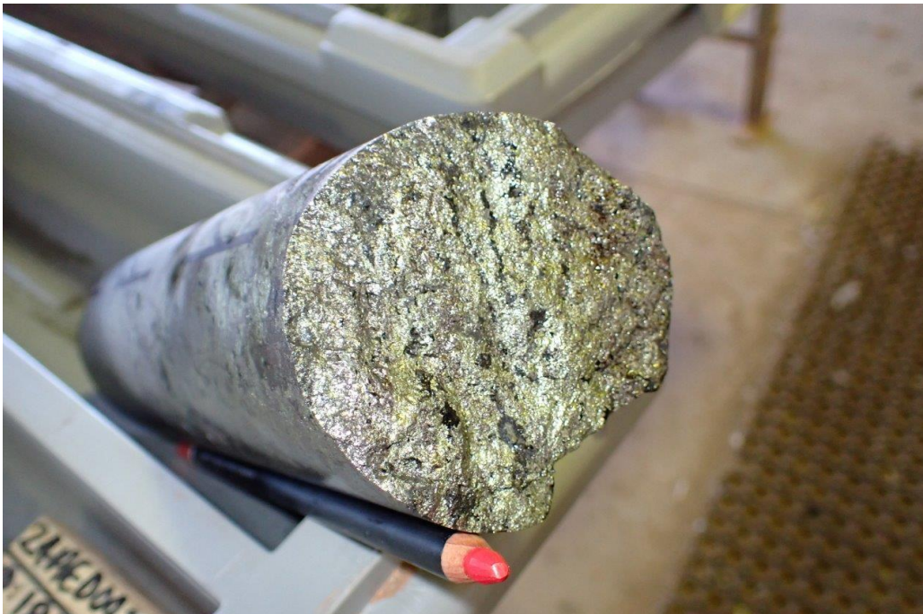
Figure 2: Massive sulphide mineralisation in 24AED002A
