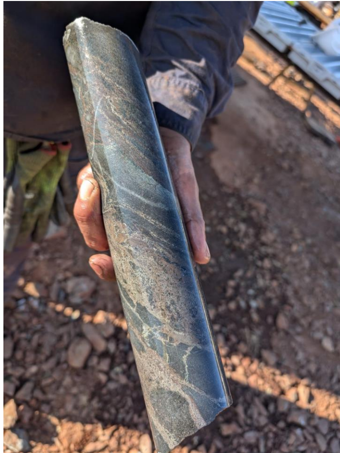
Figure 3: Sphalerite, galena and minor chalcopyrite in 24AED003
