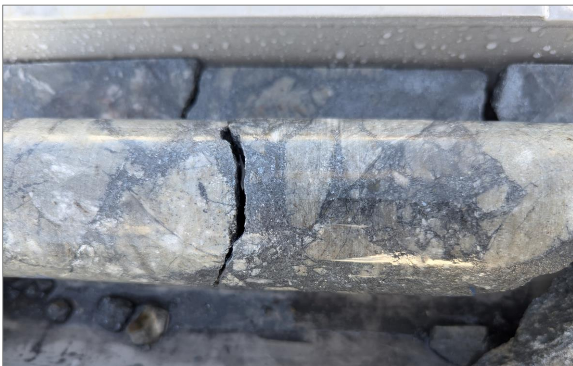
Figure 7: Core photo of the high-grade Sb interval in RDR067 highlighting brecciated ultramafic at 239.4m.
