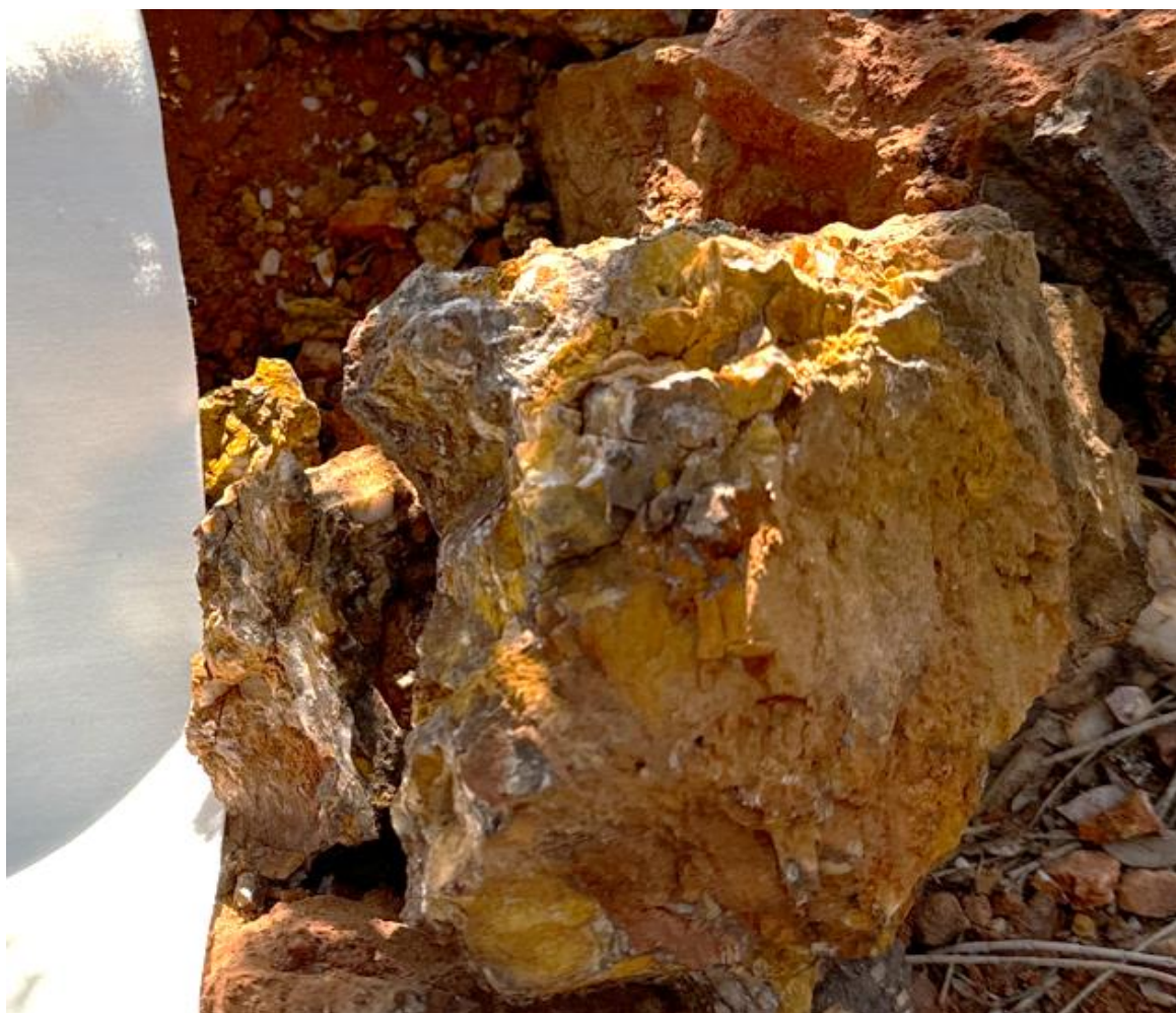
FIGURE 2: PHOTO OF ROCK CHIP SAMPLE GRADING 1.25G/T AU
