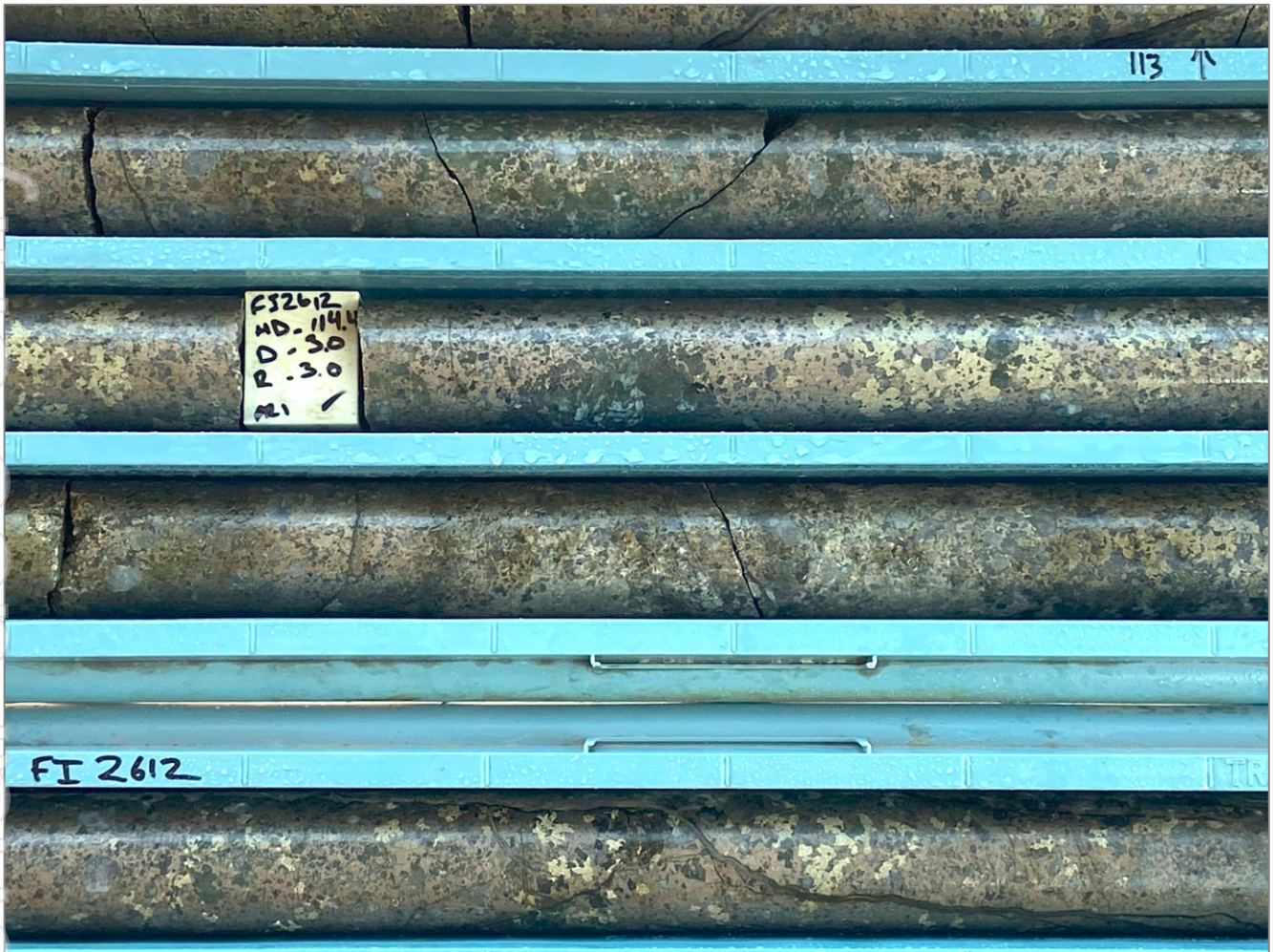
Figure 2: Detail of semi massive sulphides around 114.40 metres in FI2612 with location shown in Figure 1 above. Brown sulphides are pyrrhotite and pale-yellow sulphides are pyrite.
