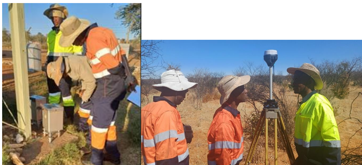
Figure 2: Gravity field crew at the Okatumba Gate Prospect setting up the Gravity Base Station and DGPS positioning.
