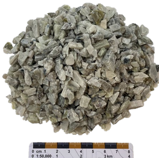
Figure 38: Final Concentrate Product Generated from the CV5 Pegmatite via DMS
