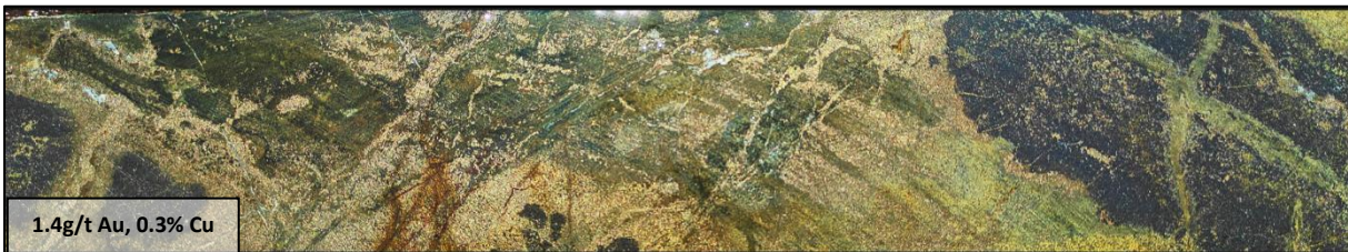
Figure 6. Core photo of gold-copper-magnetite mineralisation, 473 to 473.2m
