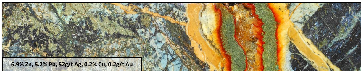
Figure 8. Core photo of breccia-hosted, epithermal zinc-lead-silver mineralisation, 528.0 to 528.2m
