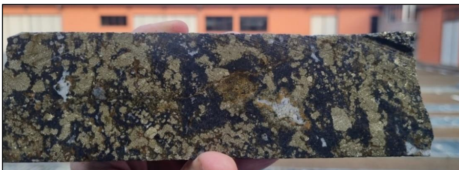
Figure 1. Core photo of copper-gold-magnetite skarn from ZRSD24150
