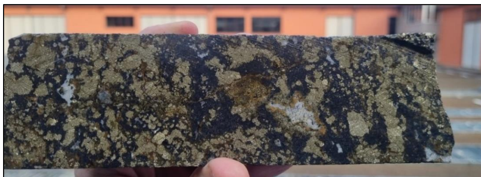
Figure 1. Core photo of copper-gold-magnetite skarn from ZRSD24150
