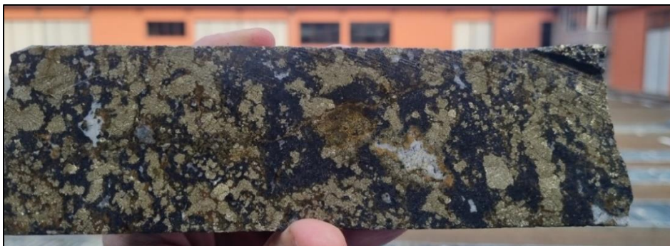
Figure 1. Core photo of copper-gold-magnetite skarn from ZRSD24150
