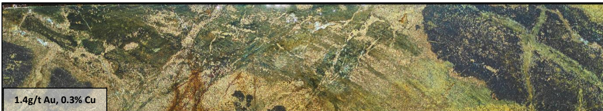
Figure 6. Core photo of gold-copper-magnetite mineralisation, 473 to 473.2m
