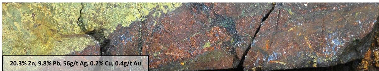
Figure 7. Core photo of massive sulphides with high-grade zinc-lead-silver mineralisation, 487.5 to 487.7m
