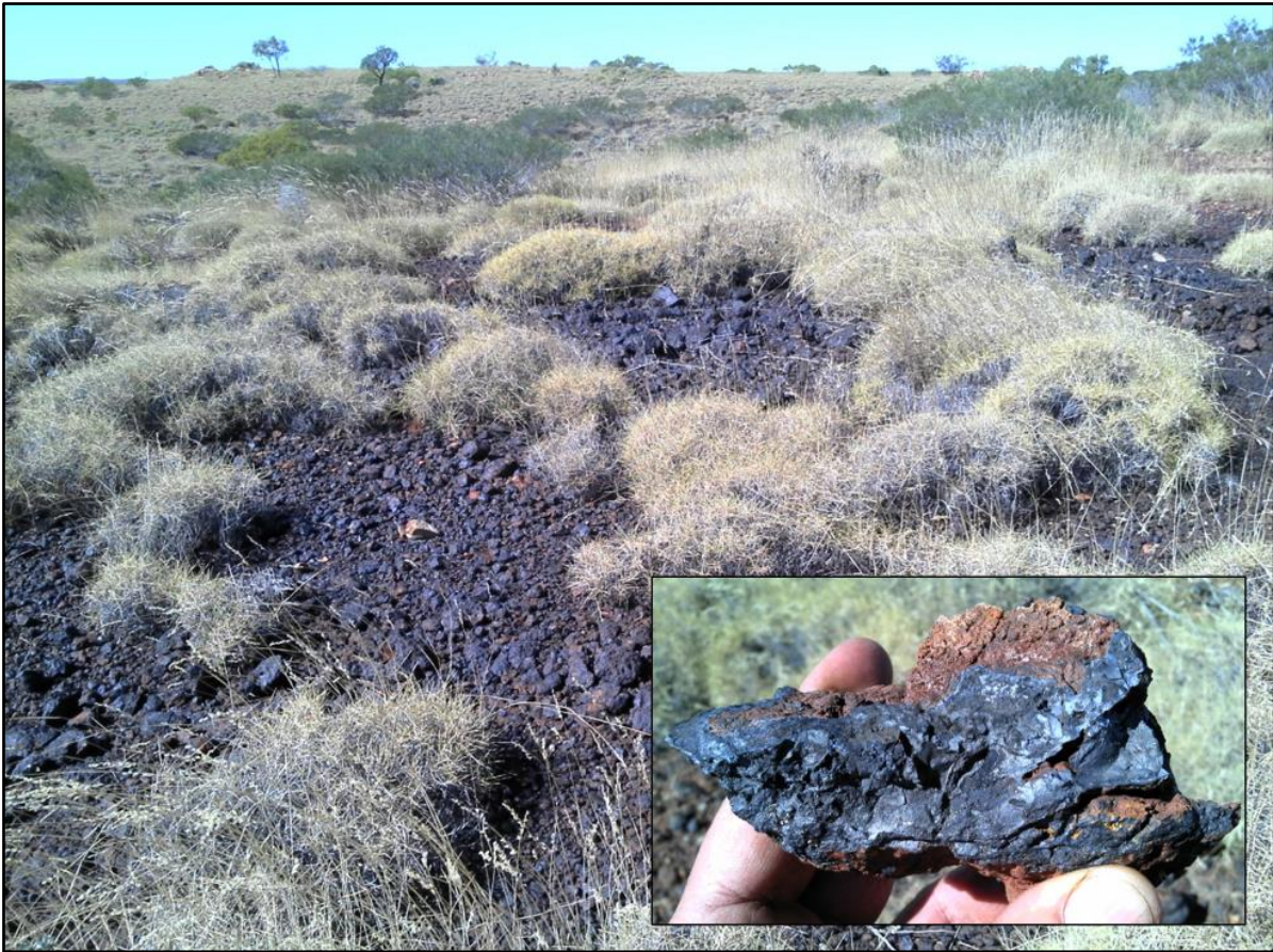
Figure 5. HD1 prospect showing manganese outcrops (looking east). Inset - manganese sample from HD1
