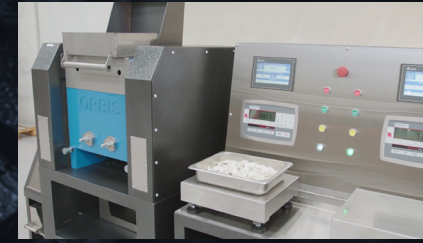
Sample Weighing Station Samples are weighed and the final sample weight is entered into the PLC
