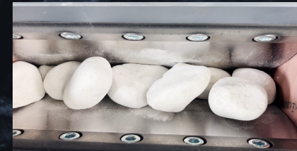
Laboratory Crusher Samples crushed from size of up to 110mm down to <2mm
