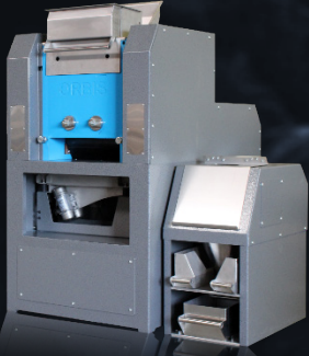
Crush raw samples
