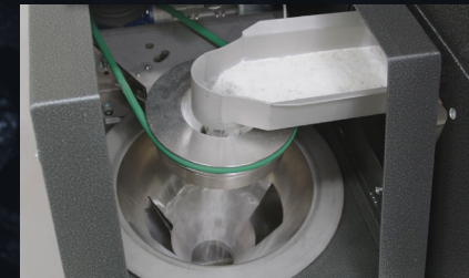
Sample Splitter Splitter automatically creates representative sample at required weight for analysis process
