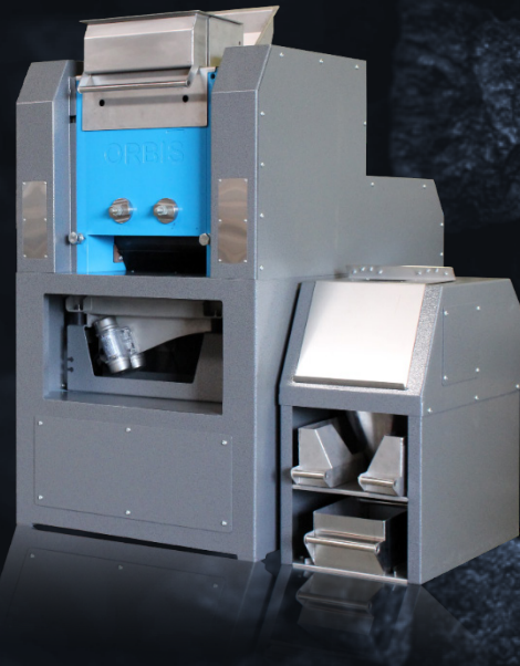
Laboratory Jaw Crushers
