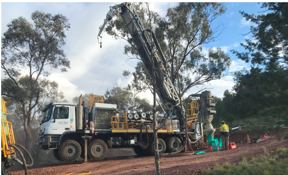
Photograph 1: RC drill rig set up at the Achilles Prospect.
