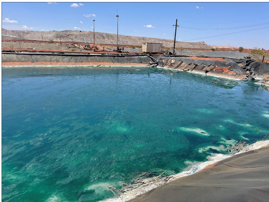
Figure 9-2: Pregnant leaching solution in pond
