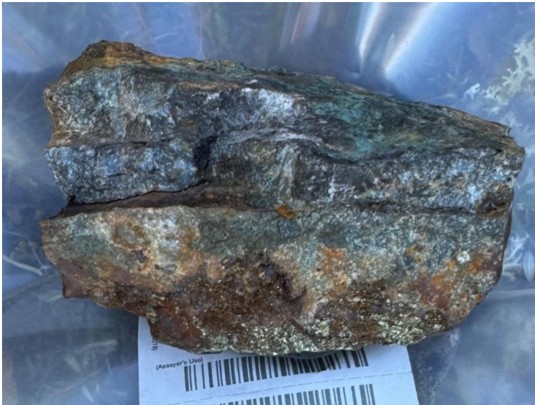
Figure 3 - Photograph of sample F005669, quartz-sulphide veining from Coyote which returned 16.95g/t Au, 45.3g/t Ag and 10.55% Cu .
