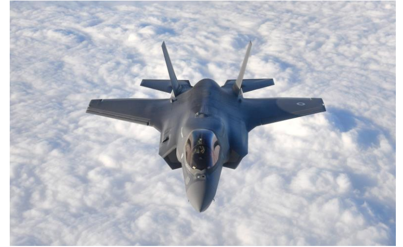
Lockheed Martin F-35 Lightning II ~20% titanium by weight
