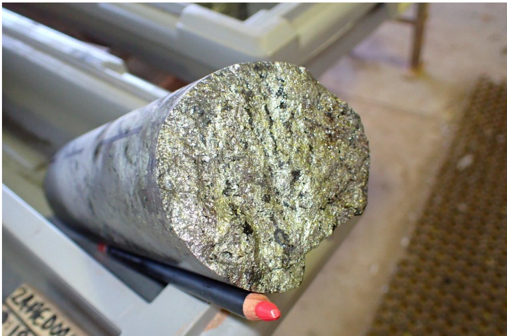
Figure 1: Massive sulphide mineralisation in 24AED002A
