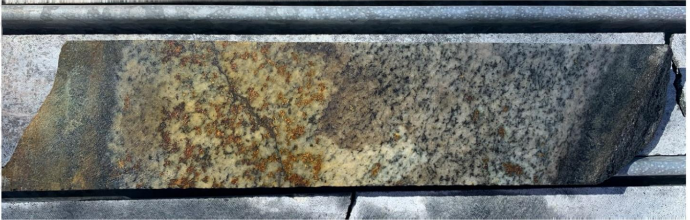
FIGURE 3: GOLD/COPPER INTERSECTION LJPD0032: 0.2M @ 2.26G/T AU AND 2.36% CU HOSTED WITHIN A COARSE GRAINED INTRUSIVE
