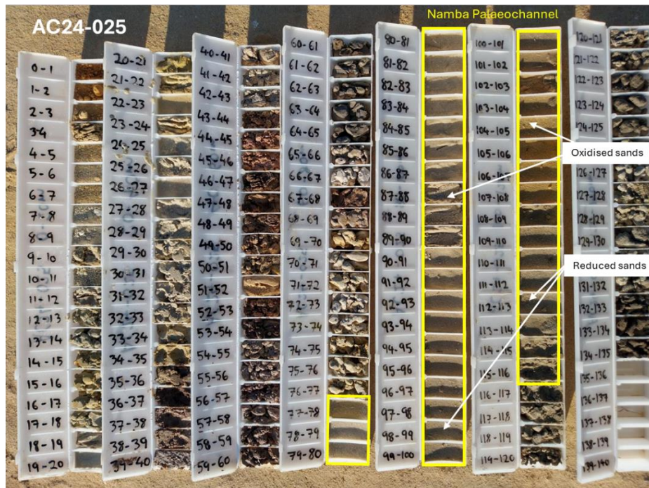
Figure 3: Chip tray samples from AC24-025 showing 39m thick oxidised and reduced Namba palaeochannel sands.
