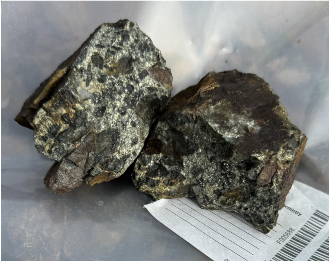
Figure 7 – Photograph of sample F005688 which returned 0.468g/t Au, 28.2g/t Ag, 6.31% Cu and 440 ppm Co from the Cleaver IOCG target.
