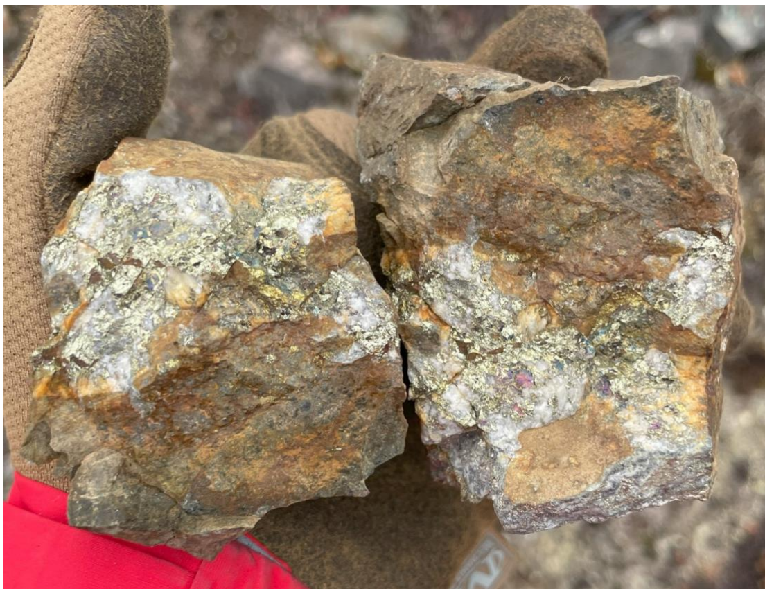
Figure 10 – Photograph of sample F005424, from a quartz-chalcopyrite epithermal vein which returned 38.2g/t Au, 76.5g/t Ag and 4.16% Cu from the Glacier Gold Epithermal Trend.
