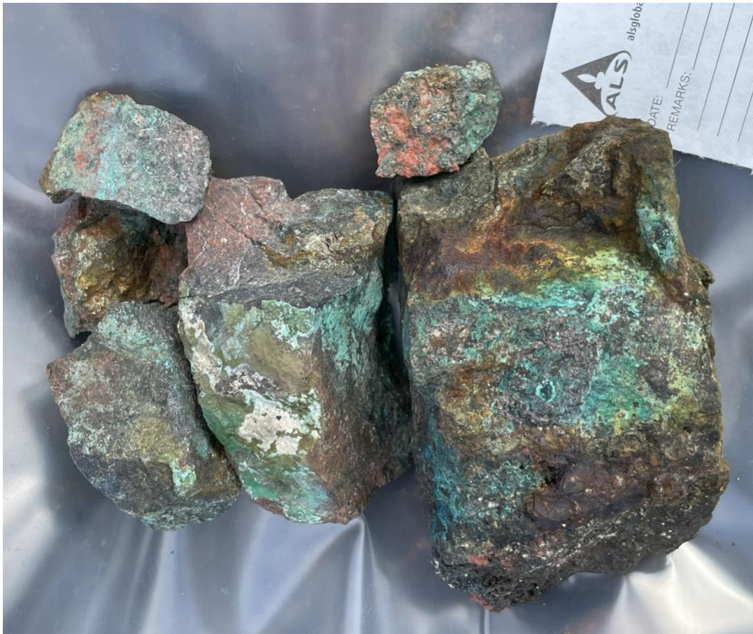
Figure 4 - Photograph of sample F005612 with chalcopyrite bearing, strongly potassic altered andesite which returned 0.615g/t Au, 11.35g/t Ag and 1.39% Cu from the west end of the Glacier IOCG target.
