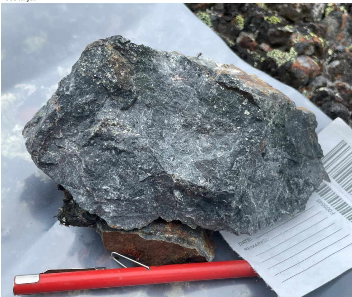
Figure 8 – Photograph of sample F005646 which returned 0.717g/t Au, 249g/t Ag, 3.0% Cu and 888 ppm Co from the phyllic altered andesite at the Cleaver IOCG target.
