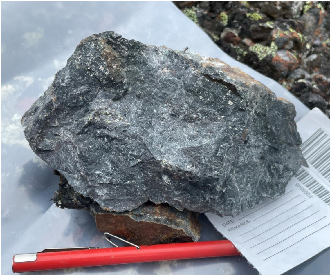
Figure 8 – Photograph of sample F005646 which returned 0.717g/t Au, 249g/t Ag, 3.0% Cu and 888 ppm Co from the phyllic altered andesite at the Cleaver IOCG target.
