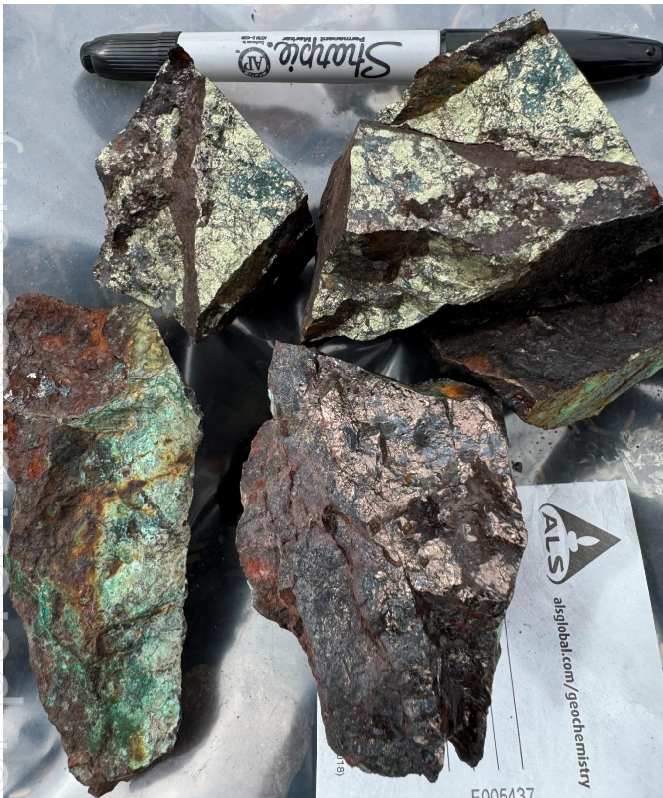
Figure 2 – Photograph of sample F005437 with massive bornite-chalcocopyrite which returned 42.60% Cu, 2.28g/t Au, 159g/t Ag, 0.364% Co from the Glacier IOCG trend.
