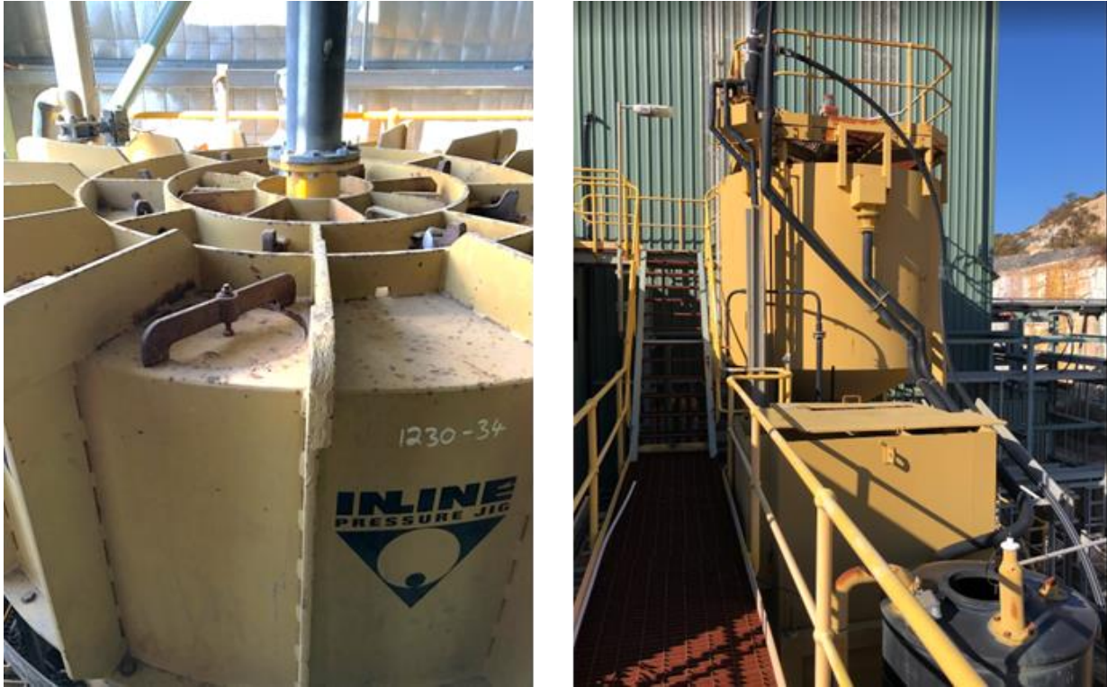
Figure 3: Photos showing the second-hand Inline Pressure Jig (left) and Intensive Leach Reactor (right) purchased by Manuka at auction.
