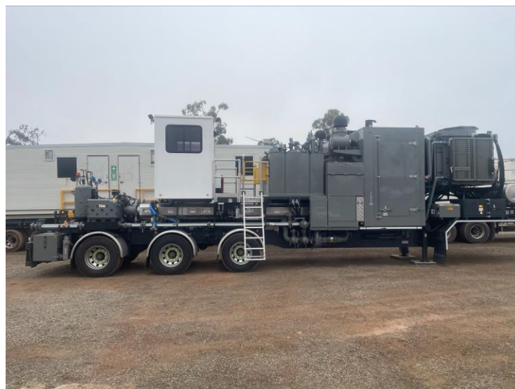
Coil Tubing Unit Cab in Miles, ready to be mobilized to the wellsite
