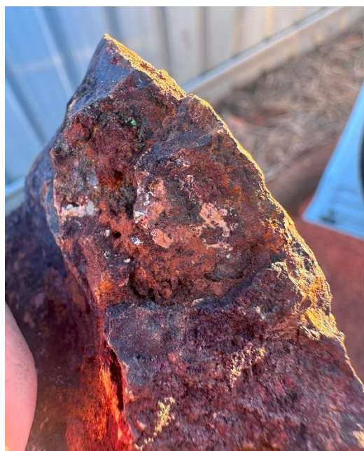
Figure 5. Sample LCV0611 showing chalcopyrite, pyrite and bornite.
