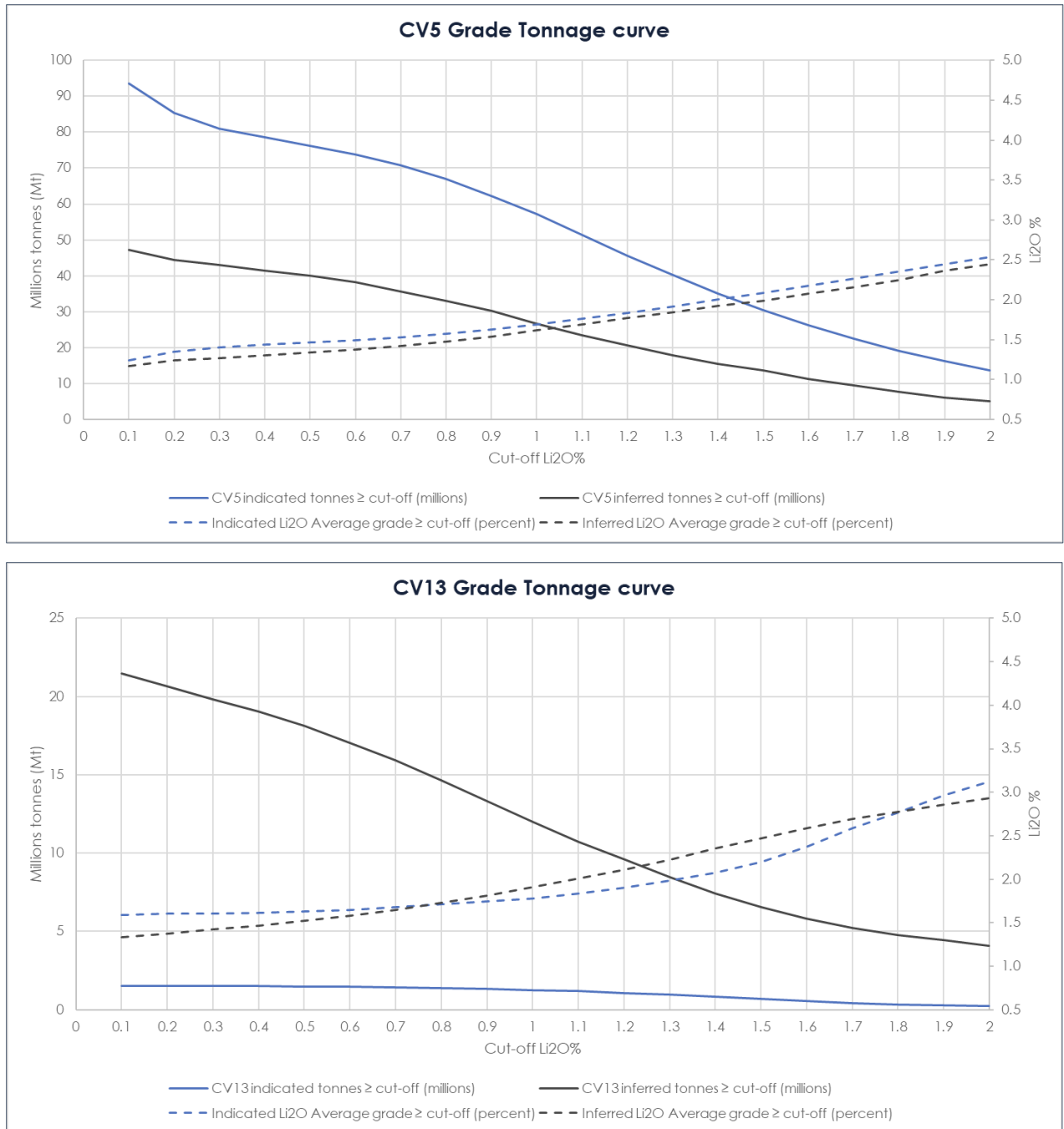
Figure 4: Shaakichiuwaanan Mineral Resource grade-tonnage curves for the CV5 and CV13 spodumene pegmatites.
