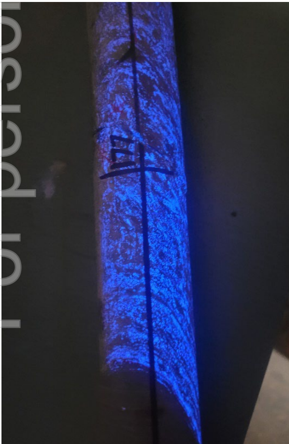
Figure 1 – WQDD013 (0.65m @ 18.35 WO 3 ) scheelite intersection under UV light
