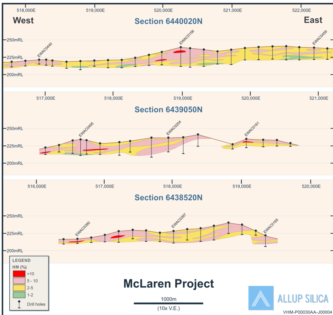
Figure 5: Cross sections from the McLaren resource illustrating continuity from surface to 35m (basement)
