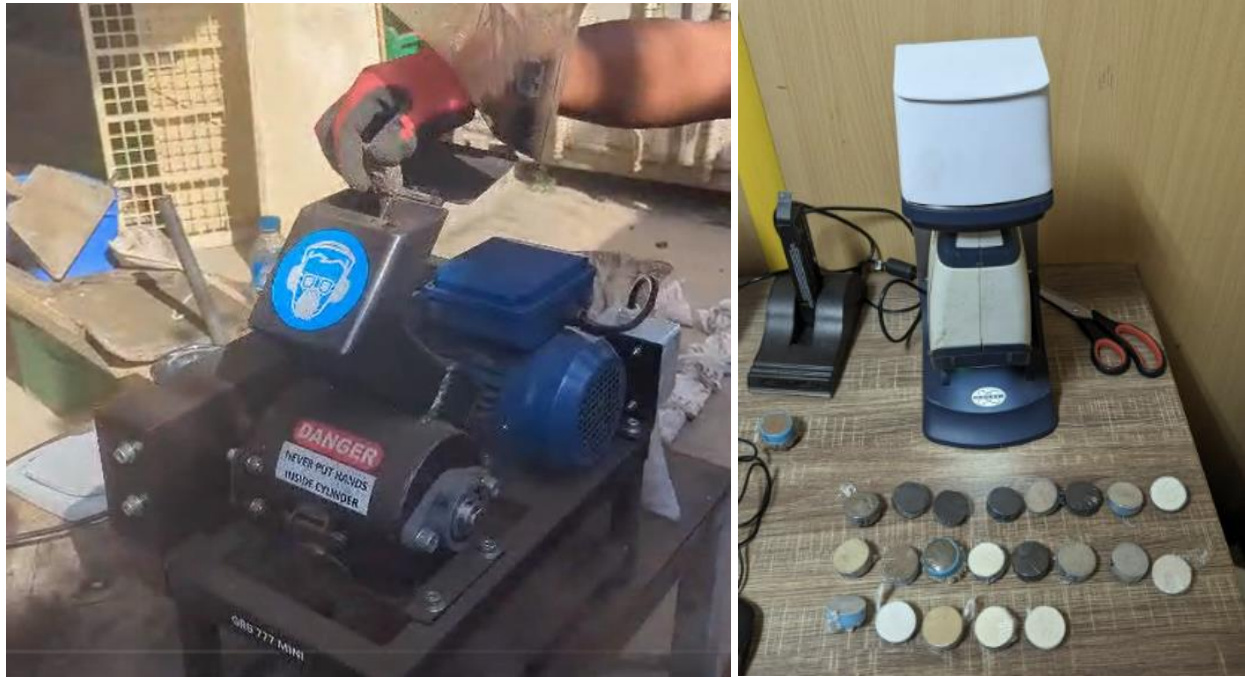
Figure 5: Crusher / Pulverisor and pXRF analysis system set up at Estrella's office in Dili with samples ready.
